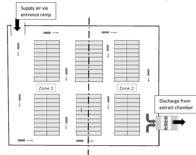
**Figure 5 – Typical ventilation system layout**
