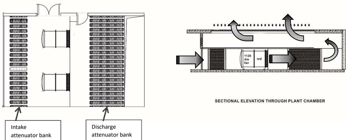
**FIGURE 3** – Creative designs are sometimes necessary to fit the attenuation into the fan chamber
