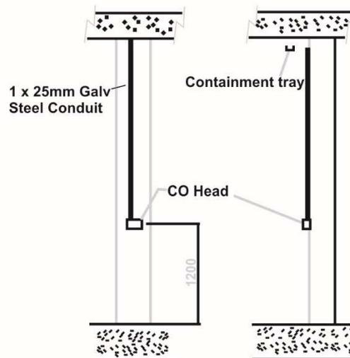
**FIGURE 2 – mounting of CO sensors**
