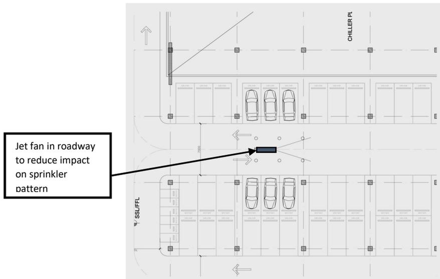
**FIGURE 10** – When a sprinkler system is installed, where possible always mount jet fans in roadways to minimise impact on the sprinklers.
