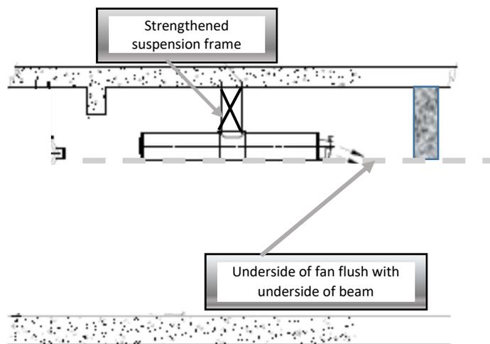
**FIGURE 8** – positioning jet fan in relation to Transfer beam & strengthened support frame
