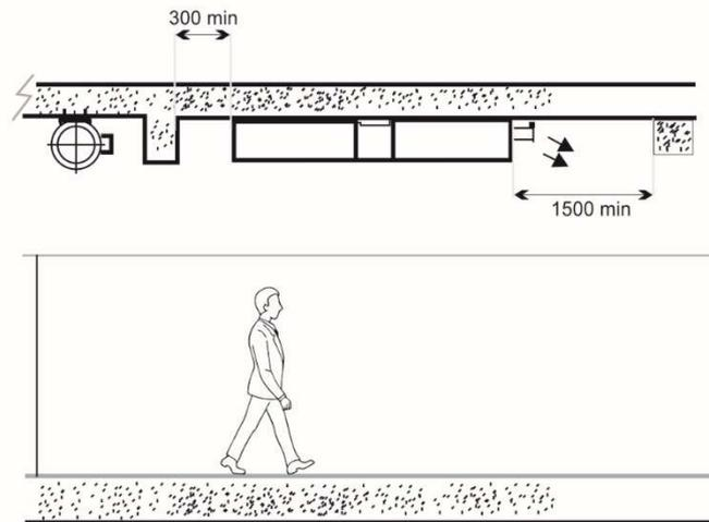
**FIGURE 7** – positioning jet fan in relation to downstand beam
